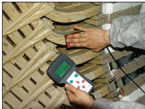
Fig. 14. Capacitance measurement for stator winding.
